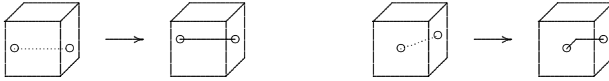
Figure 1: If the curve passes through opposite faces, it is replaced by a line segment joining the midpoints of the two opposite faces. If it passes through two adjacent faces, it is replaced by two line segments joining the midpoints of the faces via the midpoint of the cube.
